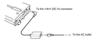
When the AC power adapter is connected to the unit, the internal battery starts charging. The  $\bigcirc$   $\bigcirc$  (power) indicator flashes during charging. When the battery is fully charged, the indicator turns off. The charging process takes about 4 hours at ambient temperature.
